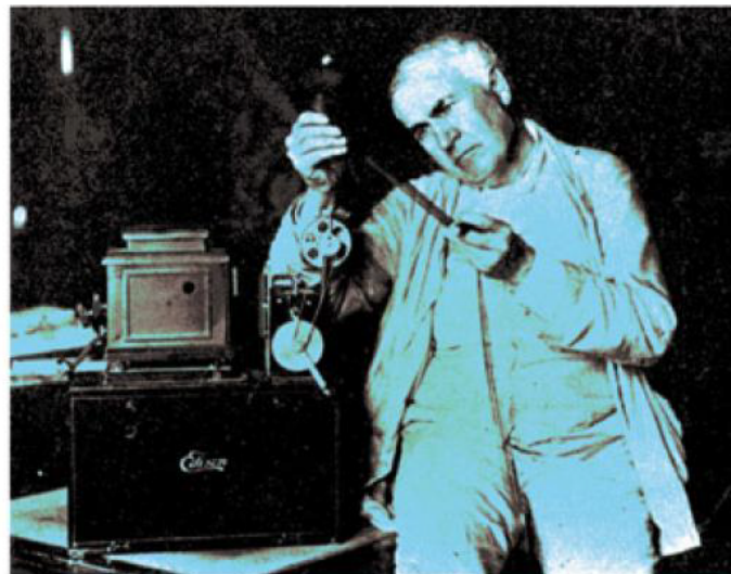
Fig. 1.7: Edison is shown here, looking over some film in the library of his laboratory around 1912. The machine is an Edison i@Home Projecting Kinetoscope. Film was passed over a magnifying glass to enlarge the pictures.
