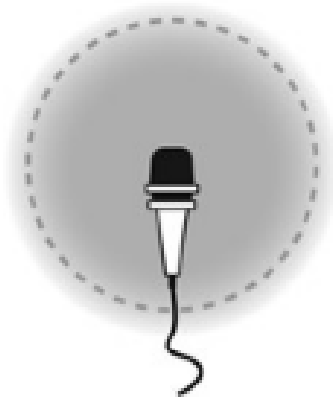
Omni-directional microphone pickup pattern
