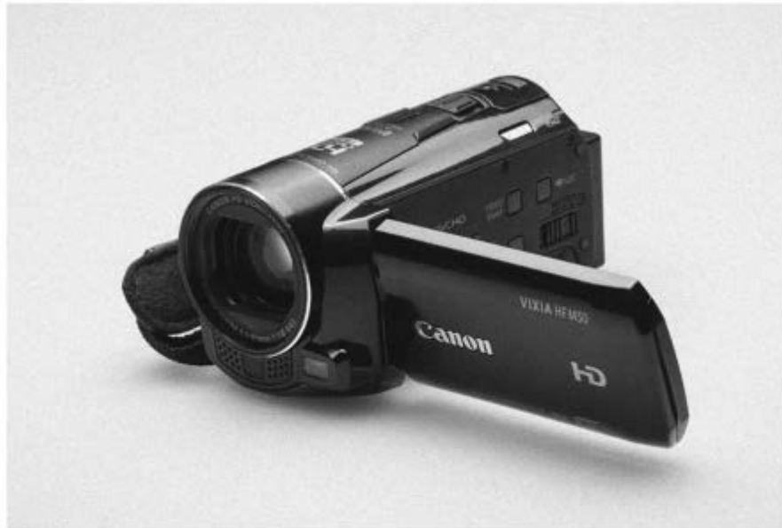
Figure 3.03 A prosumer camera has at least HD-quality video but does not have the ability to record two-channel audio with XLR inputs. (Photo by Seth Gitner)
